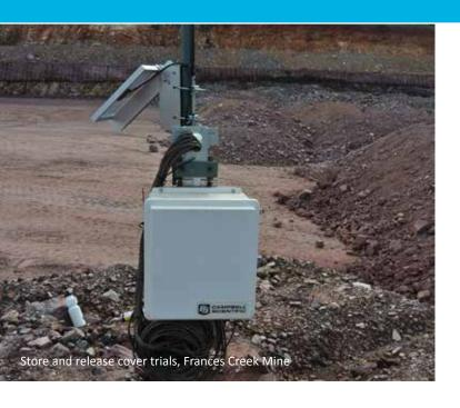
EMM is responsible for the design of the store and release covers and instrumented trials at Frances Creek Mine in the Northern Territory. The instrumented cover trials will assess the store and release cover's performance to determine if it is meeting its design intentions of being safe, stable, sustainable and non-polluting.
